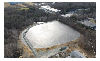
Aerial image of the Containment Area feature (engineered slurry wall and temporary cap) on the Olin property facing south, December 2021. The PRPs replaced the previous cover of the Containment Area in the fall of 2021.
